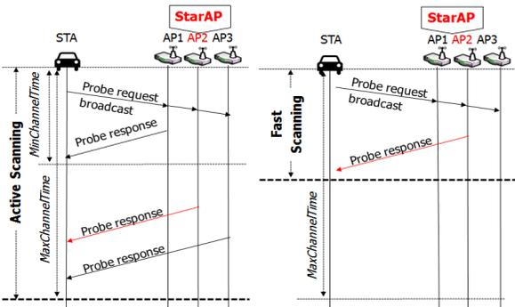
(a) Traditional scanning phase based on active mode (b) Proposed scanning phase
