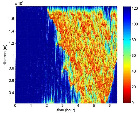
Fig. 5: Spatio temporal representation of the traffic jam (km/h)
