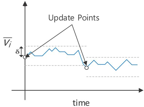
Fig. 3: Illustration of the threshold-based method
