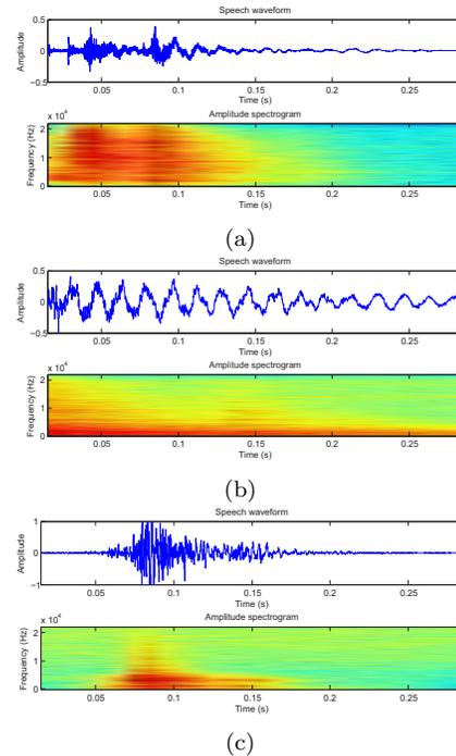
Figure 4: Sound analysis for (a) lab door (b) bathroom door (c) vehicle door
