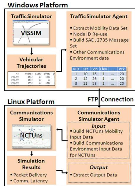
Figure 1. Proposed Integrated Simulation Framework
