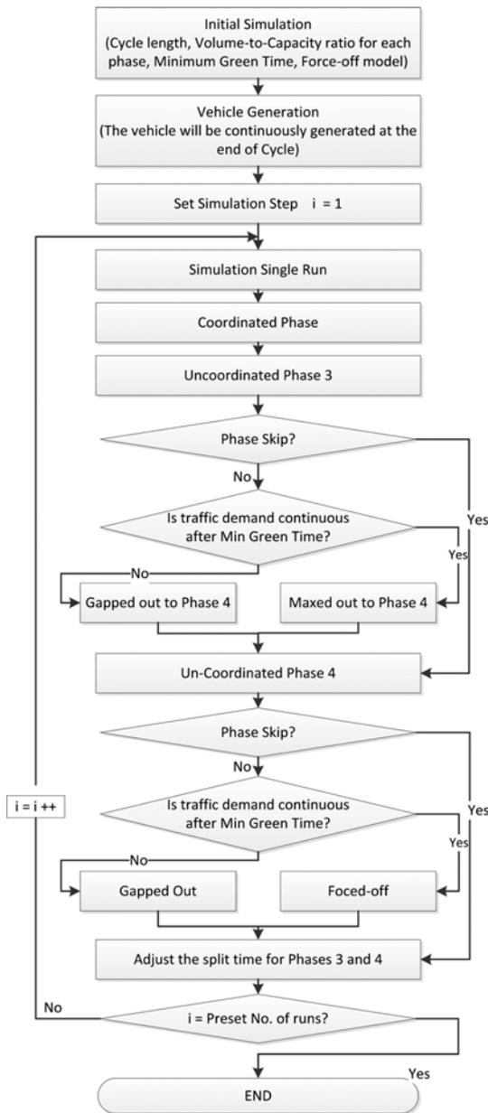
Fig. 3. Simulation Procedure of Adaptive Split Feature
