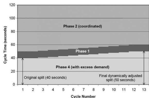
Fig. 1. An Example of Adaptive Split Feature Operation
