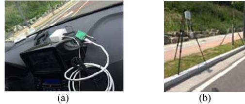
Figure 1. (a): Equipped OBU in a vehicle, (b): Deployed RSU on roadside
