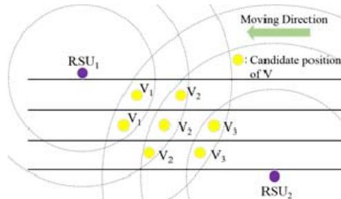
Figure 2. Estimated vehicle location through I2V communications
