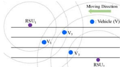
Figure 1. Measured distance from each RSU via ToA (a center of circle is RSU's coordinate and a radius is a measured distance)
