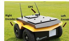
Figure 2. Unmanned Ground Vehicle Called Jackal.
