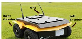
Fig. 1. Unmanned Ground Vehicle Called Jackal.
