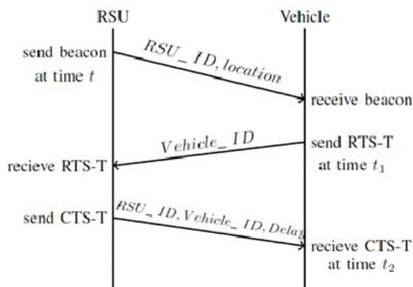
Figure 1. Time line of the two-way TOA packet handshake [3]
