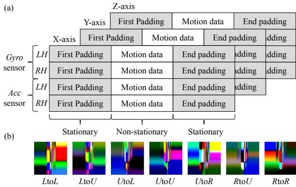
Fig. 3. Design of input data in Deep learning; (a) Input data structure (b) Example of input RGB image data after padding and re-sizing, where LH, RH, L, U, R, Gyro and Acc stand for Left Hand, Right Hand, Left, Up, Right, Gyroscope and Accelerometer, respectively
