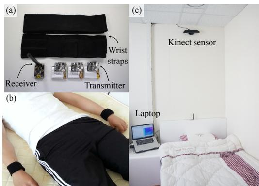
Fig. 2. System setup, (a) Sensor sets and wrist straps (b) Participant wearing wrist sensors (c) Experimental room
