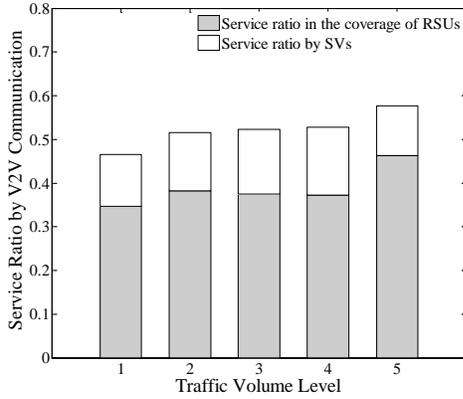
Fig. 5. Service ratio of MS by V2V communication under different traffic volume levels
