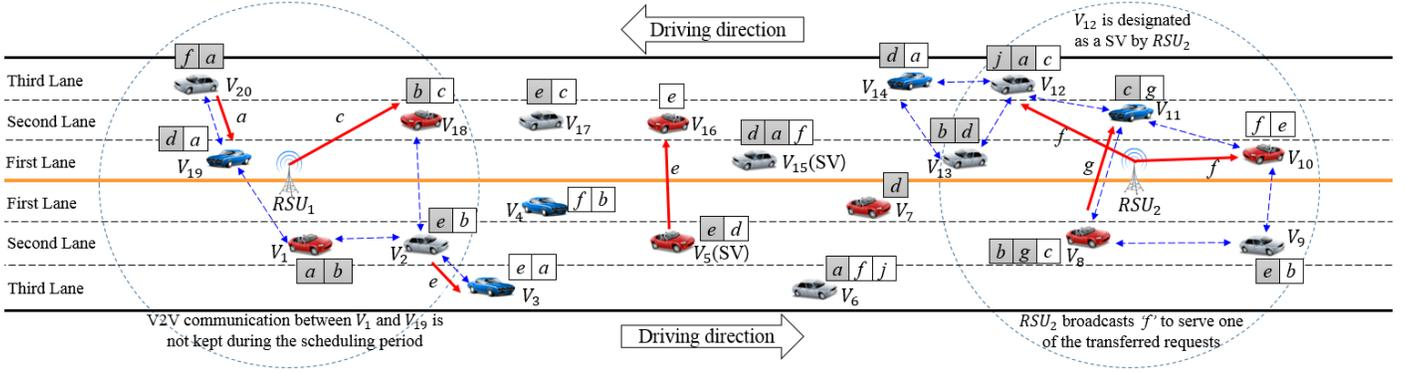
Fig. 1. Data dissemination system via cooperative I2V and V2V communications in a bidirectional road environment
