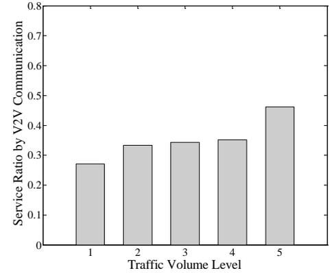
Fig. 6. Service ratio of SFR by V2V communication under different traffic volume levels
