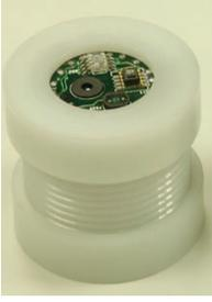
Fig. 1: Packaging using an O-ring [15][16][17]
