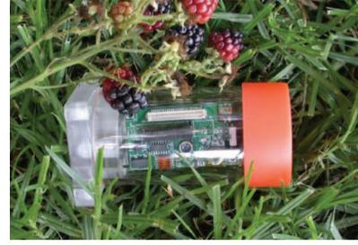
Fig. 3: Packaging using a custom-designed cylinder-shaped cover [19][20]
