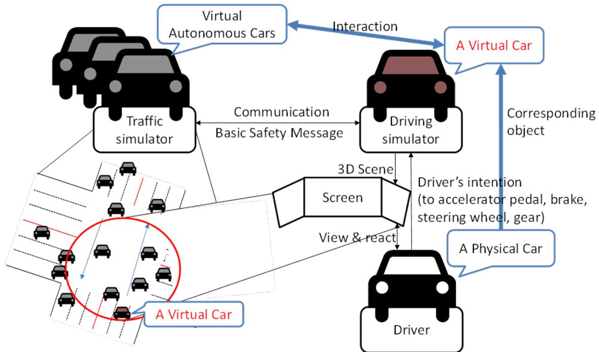
**Figure 1 – A concept of an integrated real-time interaction framework**
