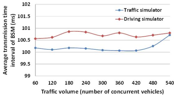
(a) Average transmission time interval of BSM as the number of vehicles increases
