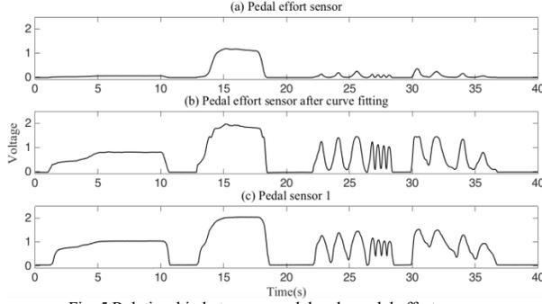
Fig. 5 Relationship between a pedal and a pedal effort sensor.
