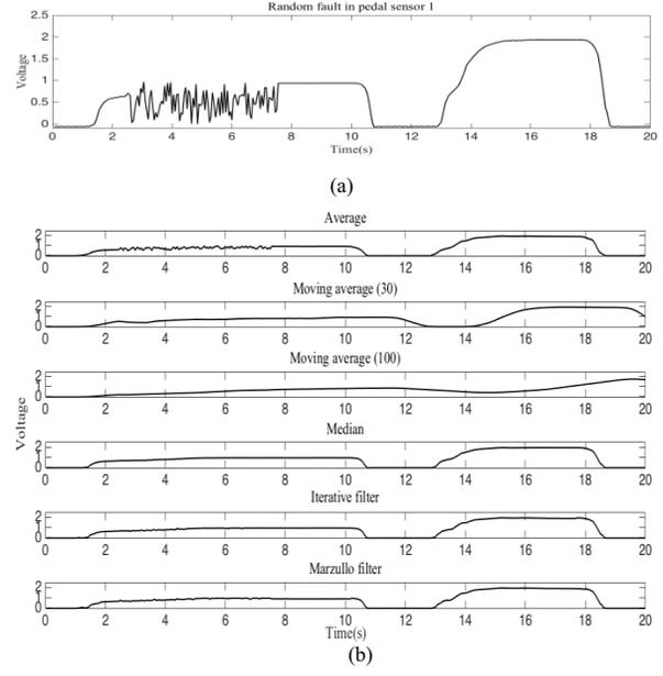
Fig. 10 Result of sensor fusion in random value fault.
