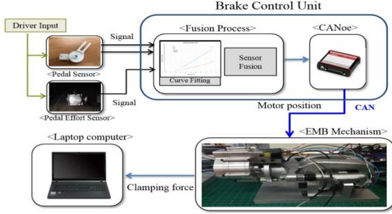
Fig. 3 EMB mechanism and the system architecture.
