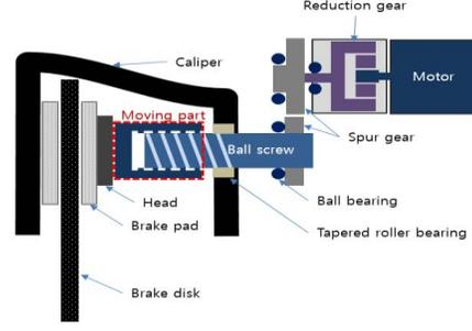
Fig. 4 Diagram of EMB mechanism.
