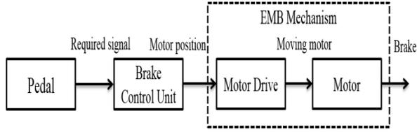
Fig. 1 General architecture of EMB systems.
