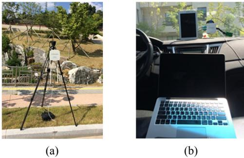
Figure 1: Devices for a field test; (a): RSU; (b): Laptop, tablet PC, and OBU.
