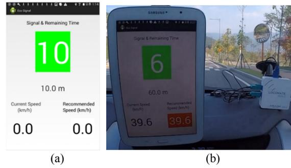
Figure 4: (a): Design of guidance application in tablet PC; (b): Screen during the field test.
